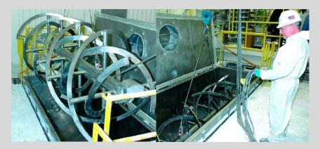
Ross Ribbon Blender with removable ribbon agitator. The ribbon is hoisted out of the blender using an overhead crane so operators can quickly and easily clean both the ribbon agitator and the trough.
